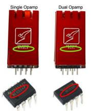
Step 3: Exercise caution while handling opamps, as they are sensitive to polarity. Plugging them in the wrong orientation can result in immediate damage. Identify the pin 1 indicator on the opamp as well as the corresponding half-moon cut on the opamp socket. Before inserting the new opamp, ensure that you have the correct orientation.
